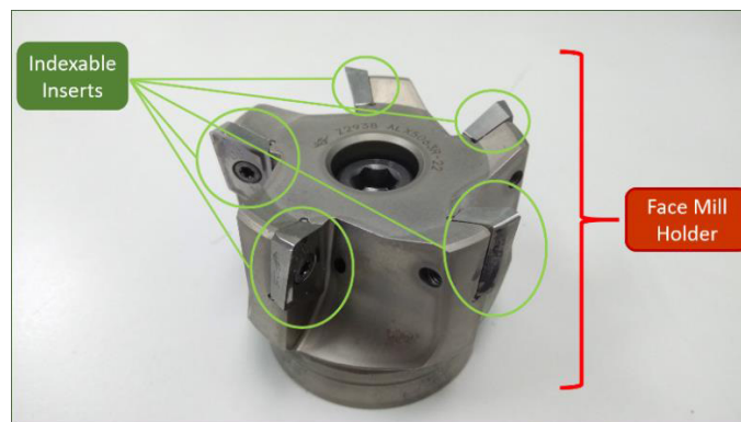
Examples of tool holders for indexable inserts
